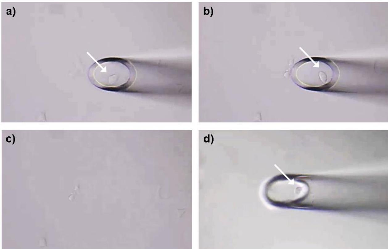
*Figure 4: HeLa cells can be selectively isolated by the MMI CellEctor. a) A single cell is chosen and approached by the micro-capillary. b) Using the Shake Mode, the microscope stage rotates and pushes the cell towards the micro-capillary, which leads to a detachment of the cell from the cell chamber. The cell can then selectively be aspirated, c) not affecting any surrounding cells, and d) finally be deposited in the target well.*
