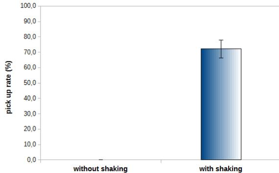
*Figure 3: Pick up rates of HeLa Cells with and without the application of the Shake Mode. Adherent single cells can be aspirated with more than 70 % success rate using the Shake Mode. Using the same conditions but not applying the Shake Mode, cells cannot be aspirated at all.*
