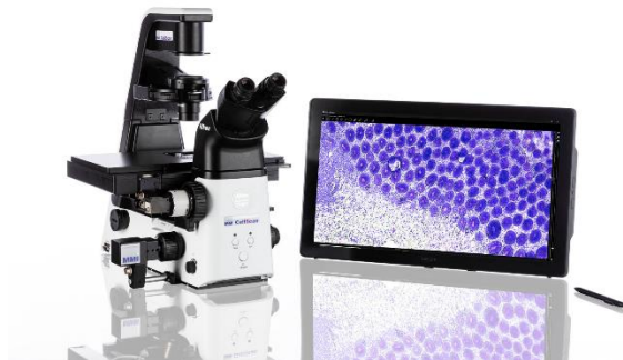
Figure 1: MMI CellScan system on the Nikon Ts2R inverted microscope. The system is compatible with many microscope brands and models and can be combined with all MMI systems for various research applications.
